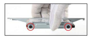
. Connect the Serial ATA and power cable to the HDD or SSD. Slide the rack into the chassis and refasten the screws.
