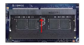
. Carefully push down the memory module until it snaps into the
