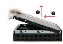
3. Unfasten the rack mount screw and remove the drive holder.
