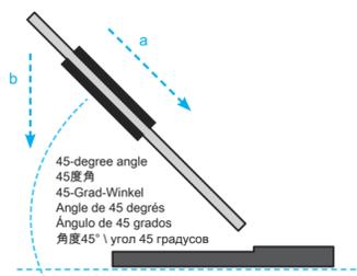
Carefully push down the memory module until it snaps into the locking mechanism.
