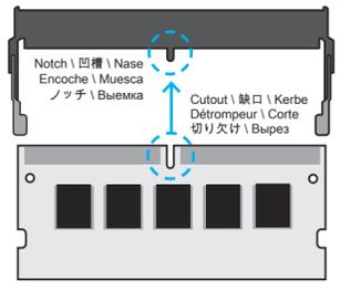
Gently insert the module into the slot in a 45-degree angle
