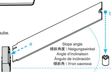
3. Slide the bracket back into the chassis and tighten the thumbscrew and two screws.
