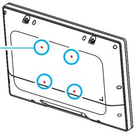
The Panel PC can be wall-mounted using a VESA compatible 100 mm x 100 mm wall / arm bracket. The maximum load capacity is 10 kg and mounting suitable in heights of ≤ 2 m only. The metal thickness of the VESA mount must be between 1.6 and 2.0 mm.
