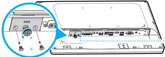
2. Install the M.2 device into the M.2 slot and secure with the screw.
