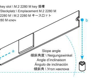
Install the M.2 device into the M.2 slot and secure with the screw.
