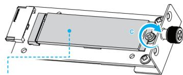
The thumbscrews should be tightened with a tool after both initial installation and subsequent access to the panel PC.
