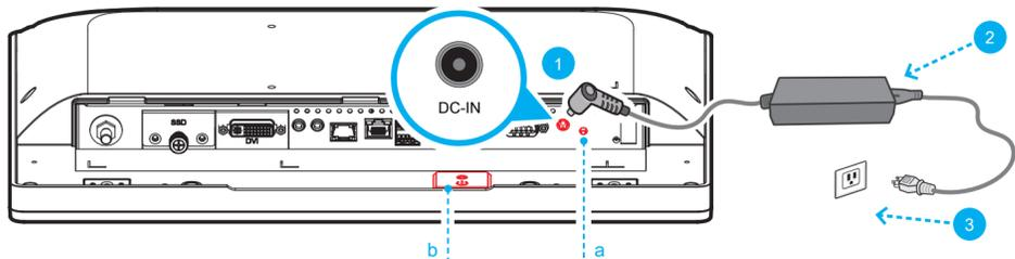
Press the power button (a or b) to turn on the system. Press and hold the power button (a or b) for 5 seconds to force shutdown.
