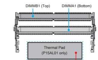
Locate the SO-DIMM and paste the thermal pad on the motherboard, which can effectively reduce its temperature. (P15AL01 only)
