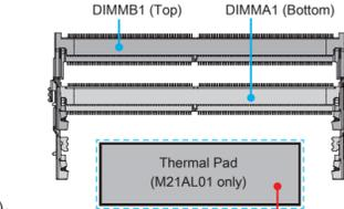
1. Locate the SO-DIMM and paste the thermal pad on the motherboard, which can effectively reduce its temperature. (M21AL01 only)
