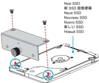
3. Slide the bracket back into the chassis and tighten the thumbscrew and two screws.
