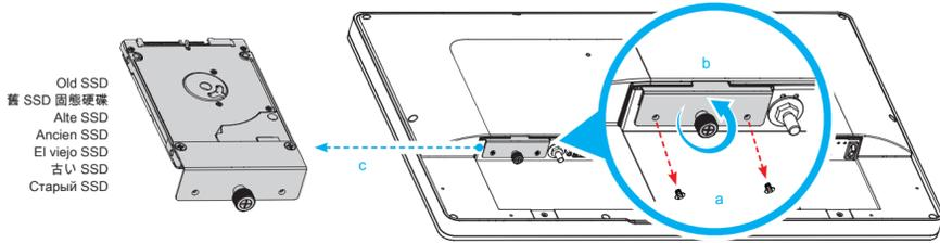
2. Unfasten the two screws (M3 x 4L) and remove old SSD.
