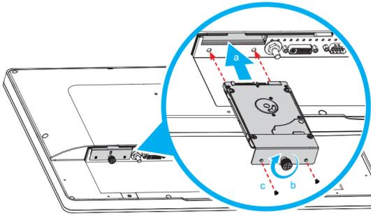
**⚠** The thumbscrews should be tightened with a tool after both initial installation and subsequent access to the panel PC.
