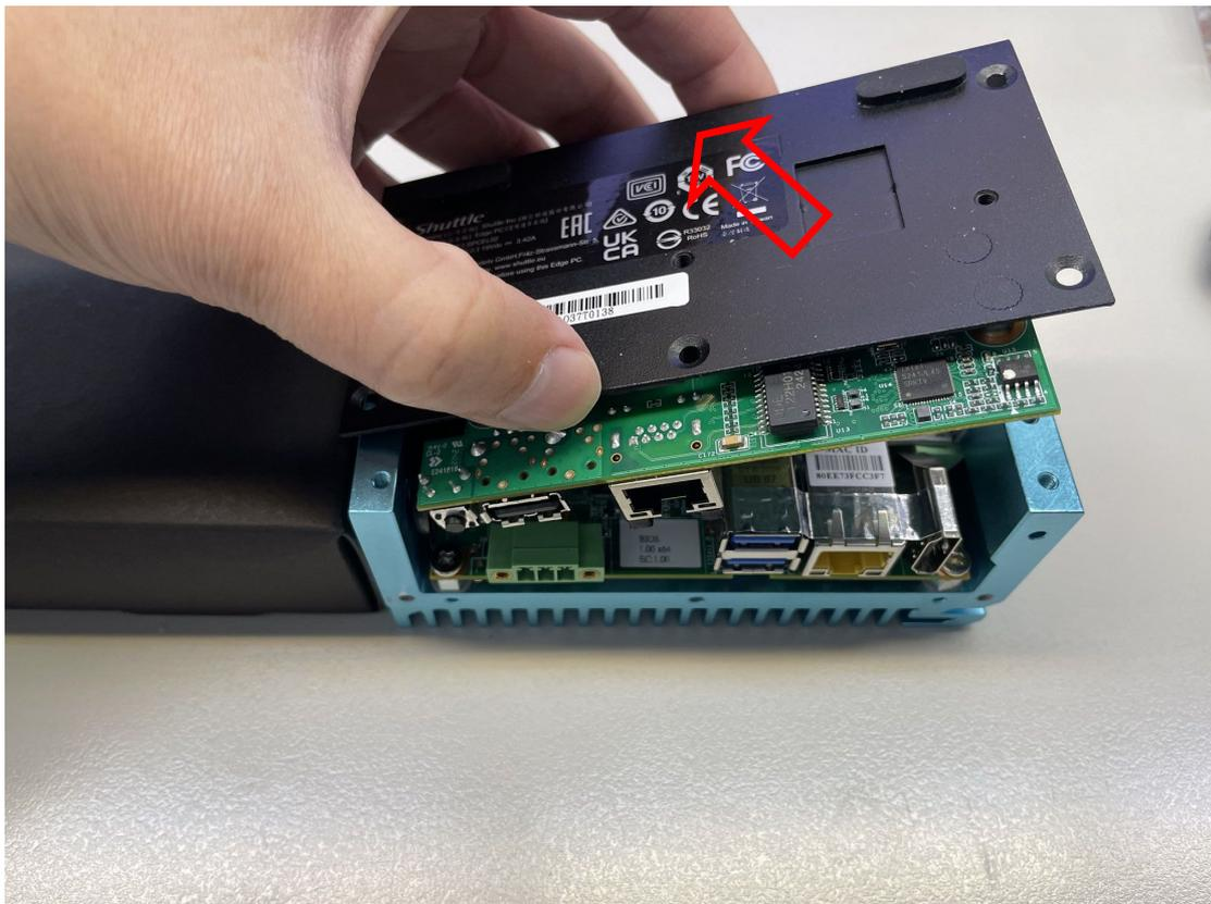
8. When opening the bottom case, do not pull the flexible cable inside.
