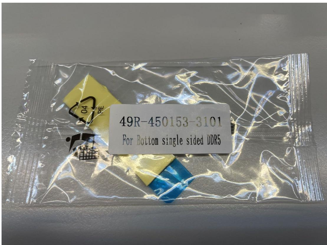
13. Remove the film from the thermal pad and stick it under the DRAM slot.
