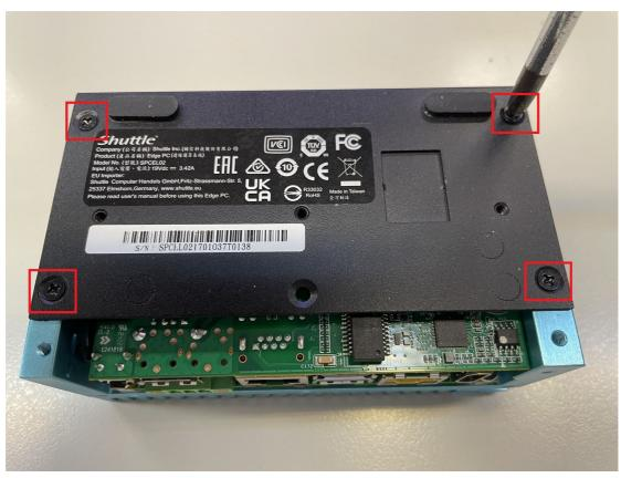
20. Tighten the 3 screws on the back IO panel
