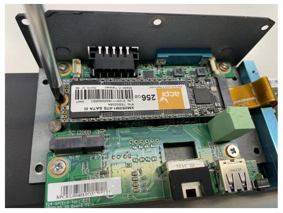
17. Install the SSD heatsink back and tighten the 2 screws.
