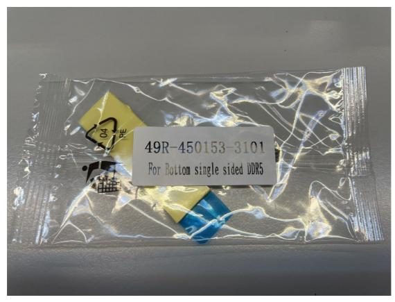
13. Remove the film from the thermal pad and stick it under the DRAM slot.
