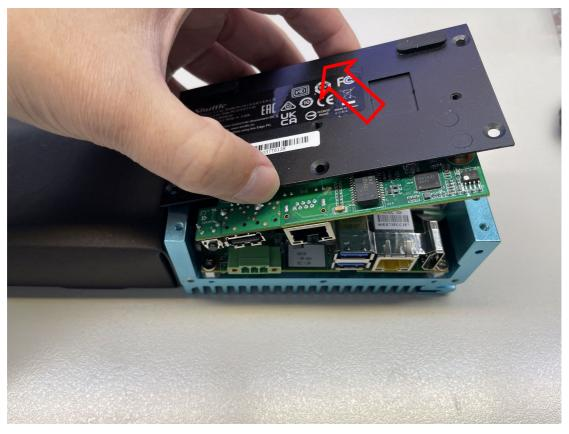
8. When opening the bottom case, do not pull the flexible cable inside.
