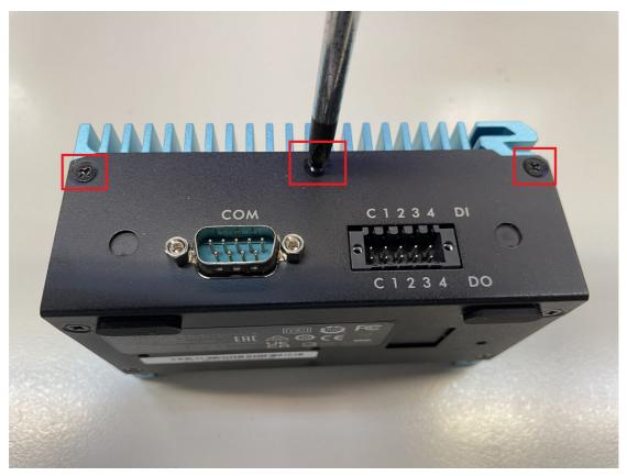
21. Push the front IO panel back into the machine and align it with the screw holes.
