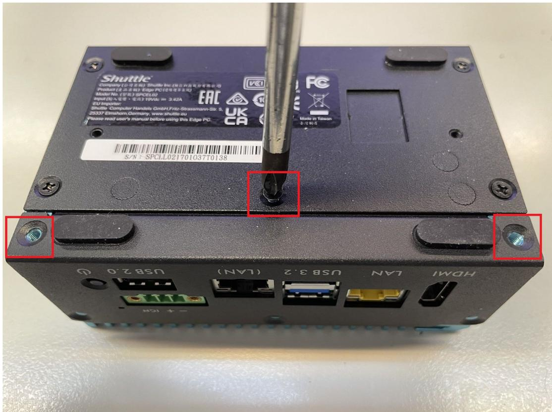
24. Tighten the last 3 screws on the front IO panel to complete the installation process.
