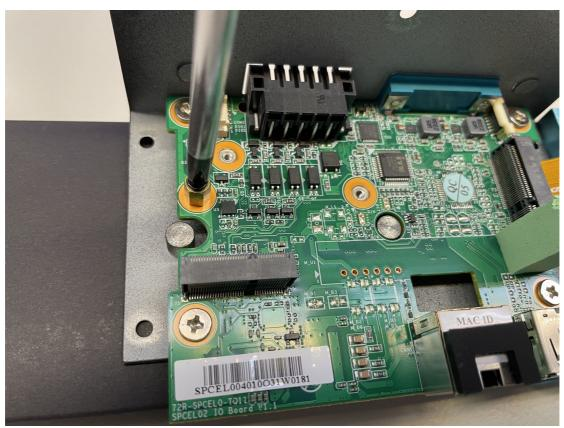
16. Install the SSD and tighten the SSD screw.
