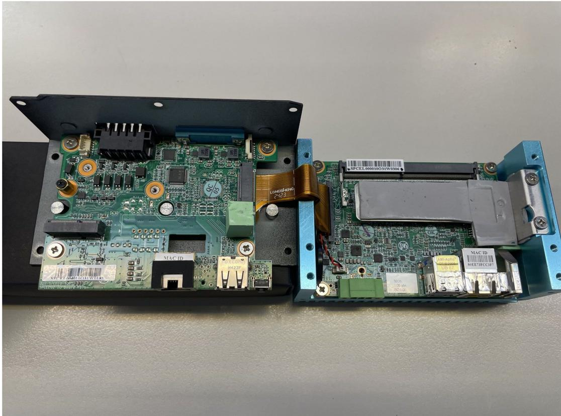
Notice: Please avoid pulling on the flexible cable when assembling components.
