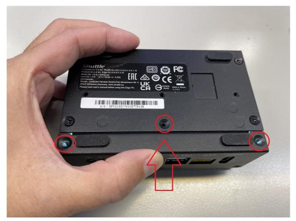
22. Tighten the remaining 3 screws on the bottom case.
